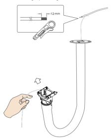
3. Fasten an intersection bracket to the side of camera. Use the included cable gland to make sure the Ethernet connection is waterproof. Pass the cable through the waterproof components, and use a crimping tool to attach to an RJ45 connector.
