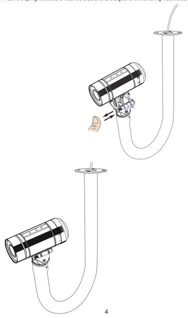
5. Secure the installation by fastening two socket screws on the other side of the camera.
