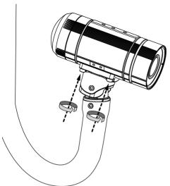
6. Loosen the socket screws on the bracket to adjust the camera's shooting direction. When done, fasten the retention screw. Please refer to the camera's documentation for more details about camera installation.
