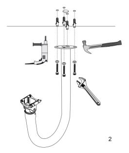
Prepare an Ethernet CAT5e cable and strip part of the cable sheath. Pass the cable through the bracket using a pull string
